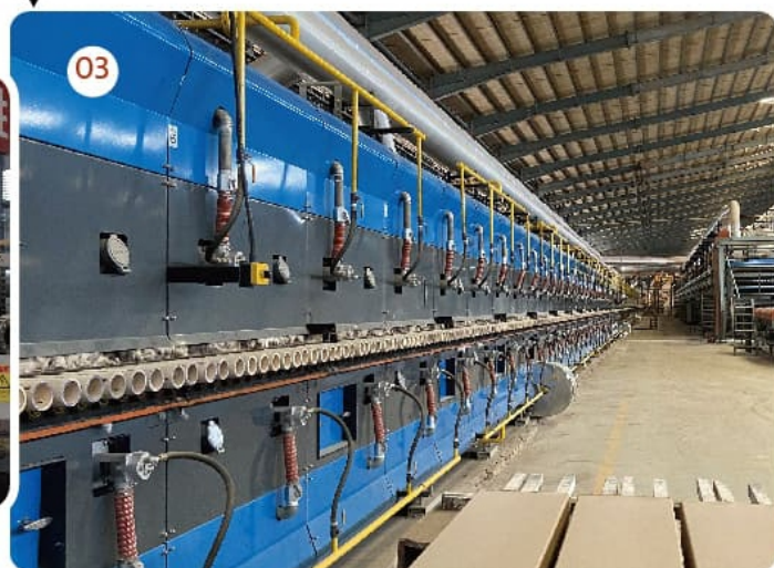
03 260 Meters Roller Hearth Kilns with Advanced Firing Systems
